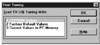
If the user has PKD-1 dongle and other than an NSM-X phone, then tuning is started automatically with EEPROM values. When using other dongles this selection opens same **Start Tuning** dialog as with TX Power Tuning.
