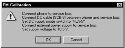
When external power is connected and user selects Yes to continue, the application displays the **Energy Management Calibration** dialog box:
