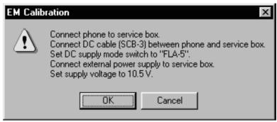
When external power is connected and user selects Yes to continue, the application displays the **Energy Management Calibration** dialog box:
